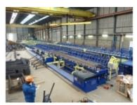
Automated shear lines for rebar cutting from USA and Europe.
